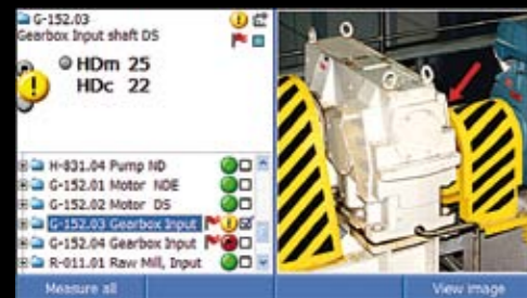
Measuring point window with photo
